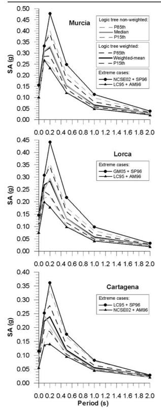
◄ Fig. 9 Comparison among the resulting UHS from nonweighted and weighted solutions of the logic tree at Murcia, Lorca and Cartagena. Maximum and minimum spectra arising from specific choices of seismic source zonings and ground motion attenuation models (extreme cases) are also shown at each city
