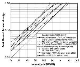
Fig. 1 Comparison among different Intensity-to-PGA conversion equations used in previous seismic hazard studies of the Province of Murcia or areas enclosing it
