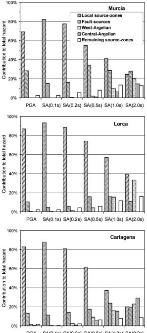
PGA SA(0.1s) SA(0.2s) SA(0.5s) SA(1.0s) SA(2.0s) Fig. 10 Contribution of seismic sources to total hazard at Murcia City, Lorca and Cartagena for the 475-year return period. See text for explanation
