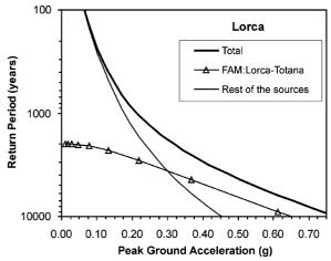
**Fig. 11** Comparison of hazard curves at Lorca considering the contribution of all seismic sources (*Total*), the Lorca–Totana segment of the Alhama de Murcia Fault (*FAM*), and the remaining sources. Note that hazard due to FAM overpass the contribution from the rest of the seismic sources at approximately the 3,500-year return period. The same results were obtained for SA(0.5, 1.0 and 2.0 s)
