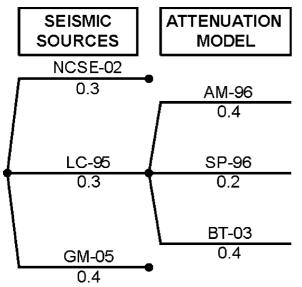
**Fig.** 7 Structure of the logic-tree considered in this study. Note the different weights on each of the branches. See text for the meaning of abbreviations
