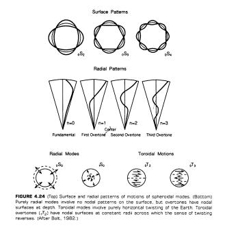
Figure 4.31: Surface and nodal patterns of free oscillations.
