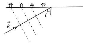
Figure 4.13: Determination of the ray with a seismometer array
