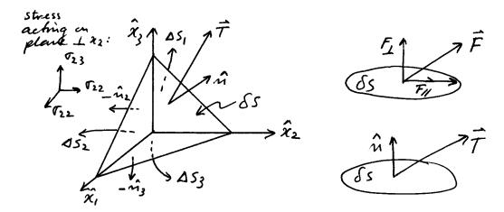
Figure 4.1: Stress balancing in the stress tetrahedron.
