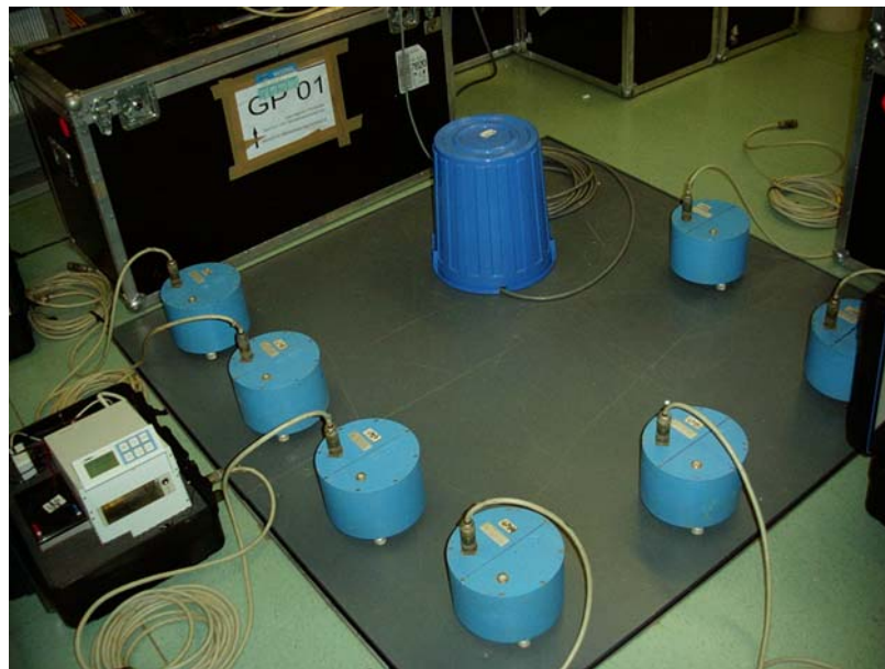
Figure 4-2 Huddle test of first seven Lennartz 3D-5s seismometers (GP01-GP07) together with the KS2000 broadband seismometer (thermally isolated below blue basket) in the laboratory installations of the Institute of Geosciences, University of Potsdam).
