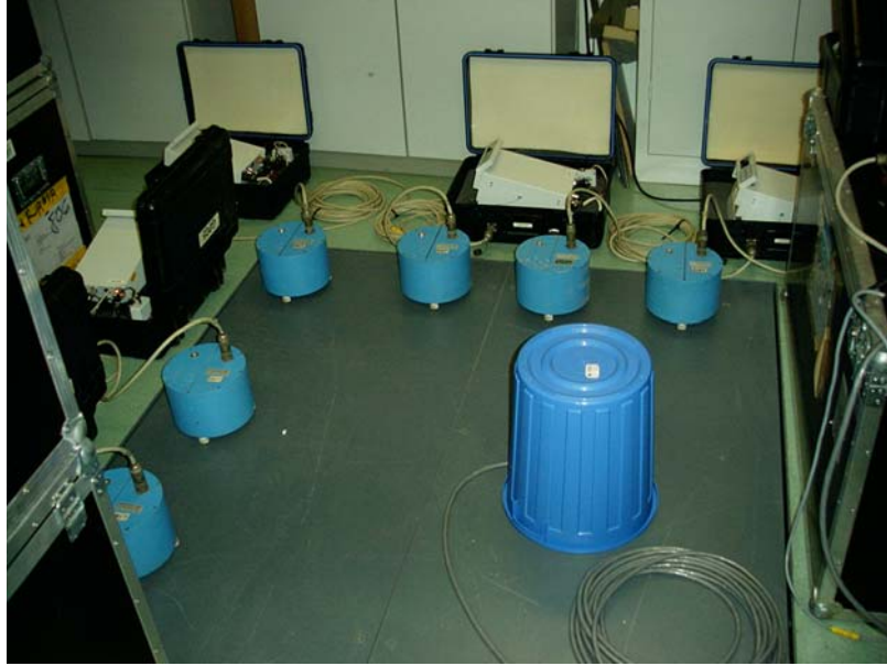
Figure 4-3 Huddle test for remaining six seismometers Le3D-5s (GP08-GP13) together with the reference instrument KS2000 (thermally isolated below blue basket).
