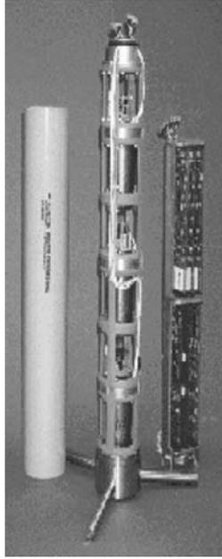
**Figure 2.47** A BB borehole sensor model KS-54000 from Geotech Instruments. The height is 2.5 m. From [www.geoinstr.com](http://www.geoinstr.com).
