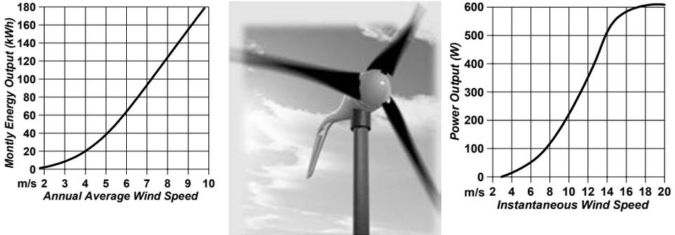
**Figure 7.16** The Air 403 wind generator. To the left is shown the monthly energy output as a function of average wind speed. To the right is shown the power output as a function of the instantaneous wind speed (Figure modified from Southwest Windpower, [www.windenergy.com](http://www.windenergy.com)).
