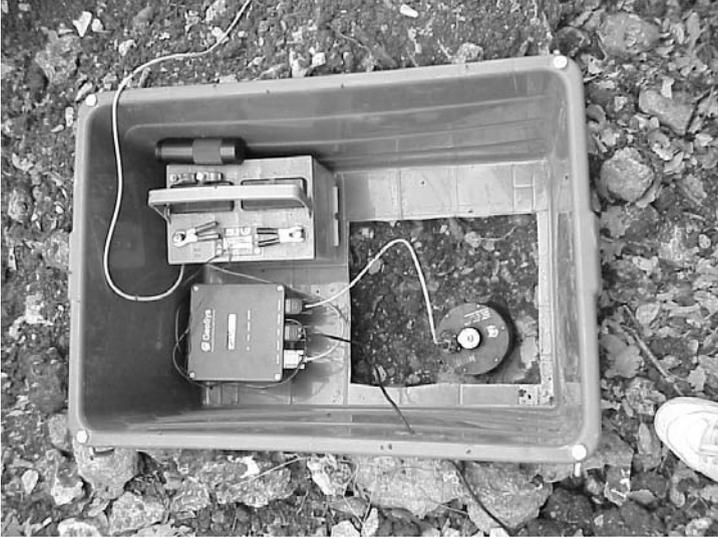
**Figure 7.12** A very simple field installation. A plastic box has been placed directly on the ground. The sensor is placed in the cut out hole. Inside are also the battery and recorder. The cable going out is for the GPS. After installation, soil was put up around the sides and insulation was put on top of the lid. The sensor is a Kinemetrics Ranger 1 Hz seismometer (Table 2.3) and the recorder is a GeoSIG GBV316 (Table 5.3).
