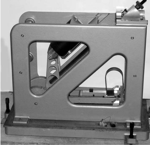
**Figure 2.18** A typical vertical long period seismometer made by Sprengnether. The cylinder seen at top center is the magnet and the coil is moving with the mass seen bottom left. Leveling is done with the 3 screws at the corners of the base plate. Once the horizontal leveling is done (back screws), the front screw is used to adjust the period. The base plate side length is 60 cm and the weight 50 kg.
