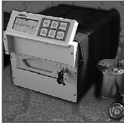
**Figure 5.11.** The Lennartz MARSliteHD recorder. Below the display is seen the 3.5" extractable hard disk. The model with magneto-optical recording is less than half the size (bottom part missing). From Lennartz home page, [www.lennartz-electronic.de](http://www.lennartz-electronic.de).
