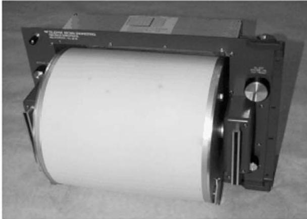
**Figure 5.4** An example of a helicorder. The unit consists of a rotating drum with paper and a pen mounted on a pen motor that translates from left to right as the drum rotates. The gain of the pen amplifier is variable to adjust to different noise conditions. This recorder is made by Geotech (Model Helicorder RV-301B). From Geotech home page, [www.geoinstr.com](http://www.geoinstr.com).
