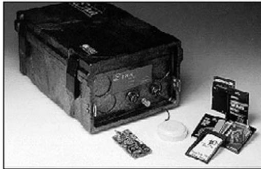
**Figure 5.14.** Example of a recorder made specifically for strong motion, the Kinematics Etna. The round white box in front of the recorder is the GPS antenna and the PCMCIA cards are seen to the right. From Kinematics home page [www.kinematics.com](http://www.kinematics.com).
