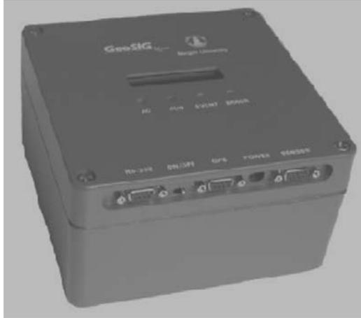
**Figure 5.12** The GeoSIG compact seismograph with 3 built in 4.5 Hz sensors. Note the standard computer connectors. In the middle on the lid is located a display giving alphanumerical information and 4 LED's give operational information. This is the most compact complete seismograph on the market. Figure made available by Christoph Kündig, GeoSIG.
