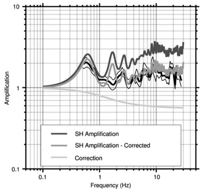
▲ **Figure 4.** Example of correcting the elastic amplification from SH-wave transfer function modeling at the SSMNet station SCUG to the common reference by applying the proposed correction function. Comparison with the ESM amplification function proposed in this paper (black).
