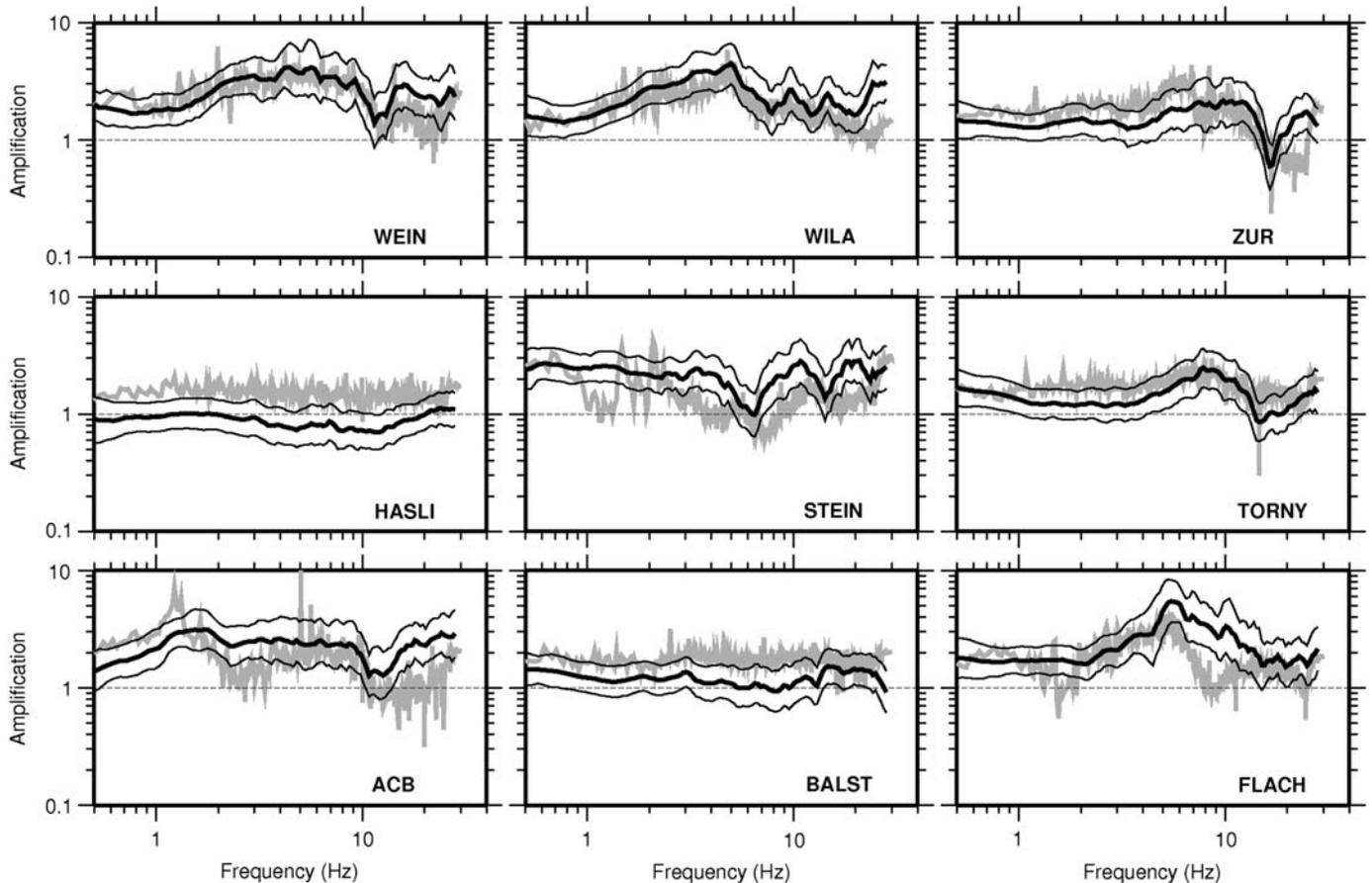
▲ **Figure 6.** H/V ratios for nine selected sites of the SDSNet compared with the elastic ESM amplification. The gray line shows the H/V derived from the ambient noise field using classical polarization analysis, the black line shows the elastic ESM amplification derived from earthquake recordings with corresponding standard deviation (thin black lines).
