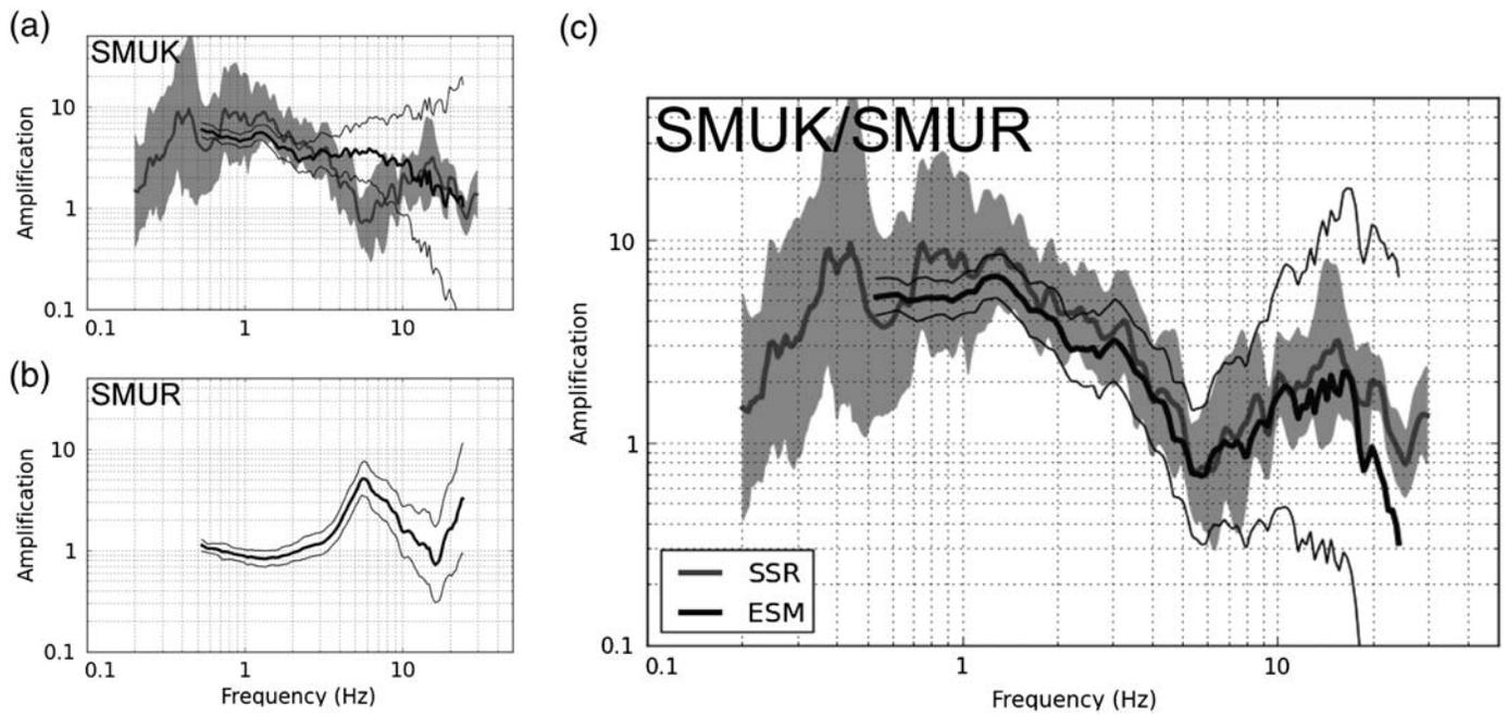
▲ **Figure 2.** (a) Standard spectral ratio SMUK/SMUR (gray) compared to ESM amplification at site SMUK (black). (b) ESM amplification of the reference site SMUR. (c) Comparison of the SSR SMUK/SMUR (gray) with the ratio of the ESM amplifications (black) between site and reference (SMUK/SMUR) finally selected for comparison.
