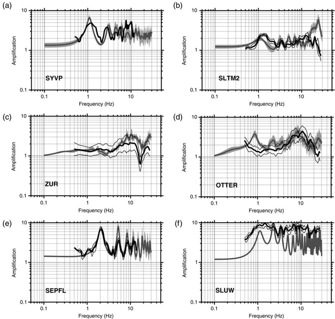
▲ **Figure 5.** Comparison of elastic ESM amplification functions from broadband spectral fitting (black line) and reference corrected elastic *SH*-wave transfer function modeling (in gray) at six test sites in Switzerland. Uncertainties are also shown, when available.
